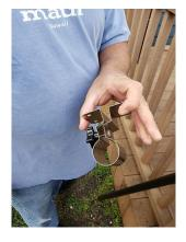
4) Insert the pole of the umbrella through both Deckhands<sup>™</sup> clamps making sure the orientations are the same. Tighten the knobs moderately. Consider which side you prefer the knobs to face. Many umbrellas have a removable lower pole section. It is recommended to have at least 21.5 inches between the upper and lower Deckhands<sup>™</sup> clamps. More is better.
