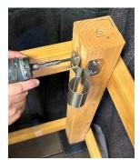
Reassemble the Deckhands<sup>™</sup> clamps, squeeze clamp together, reinsert the bolt, and tighten knob to reassemble. Reinsert the pole and hand tighten the knobs.
