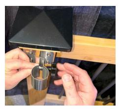
17) Tighten the slot side screws, and optionally back off 1/4 turn at a time until the Deckhands™ clamp slides smoothly when the knob is loosened. A manual screwdriver is recommended.
